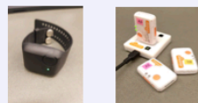
Fig. 2: The Empatica E4 wristband used to take physiological measures (left), and the Shimmer3 IMU used to measure body acceleration (right).
